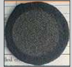
After abrasion test >8000 cycles without breaking the material
