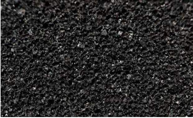
Supergrip sandy finish surface magnification
